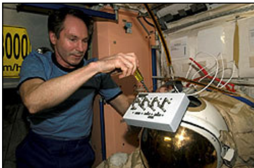
Aboard the International Space Station, Expedition 12 flight engineer Valery Tokarev puts some finishing touches on SuitSat. The flexible portion of the VHF ground plane antenna and the feed line are visible above the helmet. [NASA Photo]
